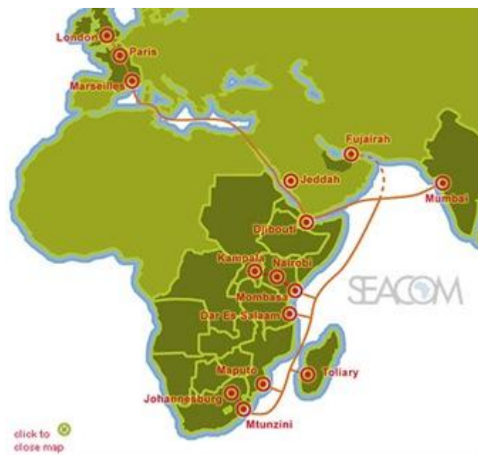
Figure 2 – The SEACOM cable and the landing stations in Africa (Source: SEACOM)
